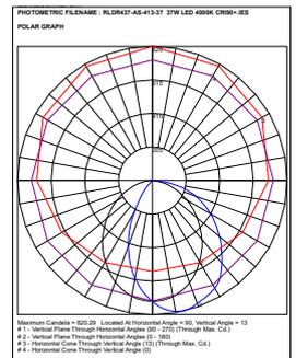
Lumen output based on Absolute lumens, 4000K LED chip and manufacturers rated mA drivers.
