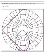
Lumen output based on Absolute lumens, 4000K LED chip and manufacturers rated mA drivers.
