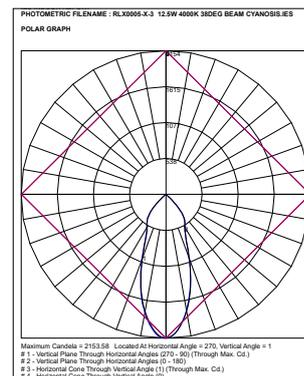
Lumen output based on Absolute lumens, 4000K LED chip 38° beam angle and manufacturers rated mA drivers.
